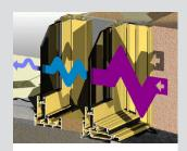
For serious sound reduction, use Vantage SoundOUT™. In some cases, the Vantage SoundOUT™ window may perform better than the wall it is being built into.
