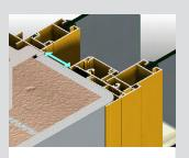
Installing this product will create a thermally broken double glazed door that will significantly reduce heating and cooling costs.
